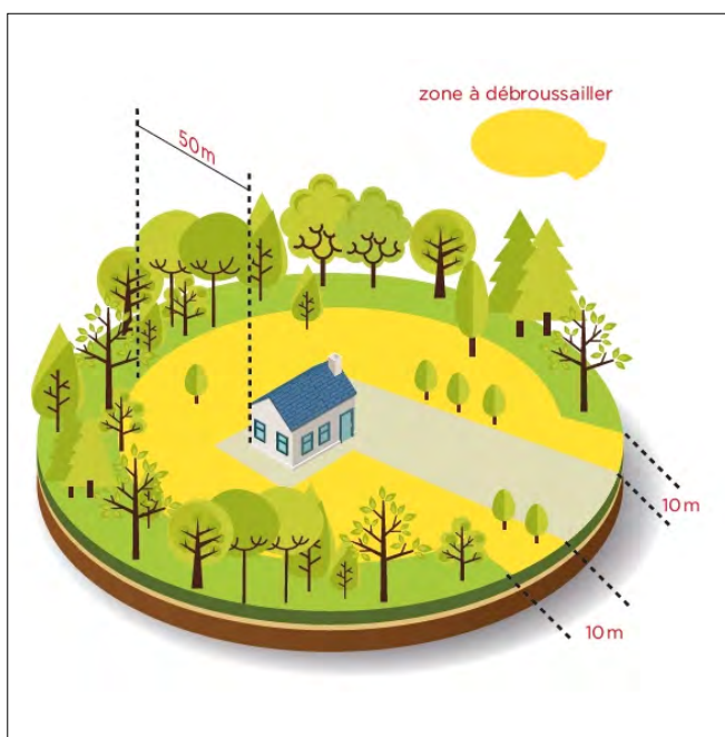
Figure 2. Compulsory brush clearing strips around buildings and access roads in France (© Mairie de Saint Christol lez Alès).
