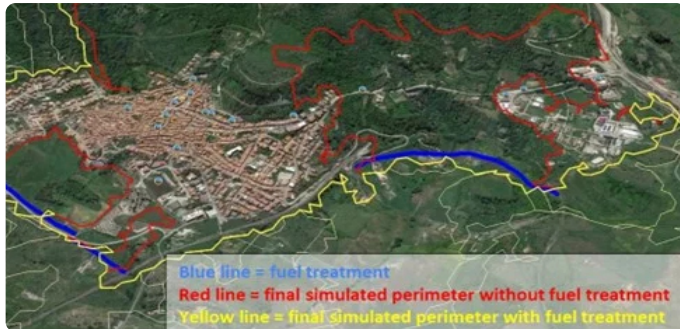
Figure 1. Simulator output used to tailor fuel treatments. If fuels on the blue lines are eliminated the area between the blue and the red lines is not burned.
