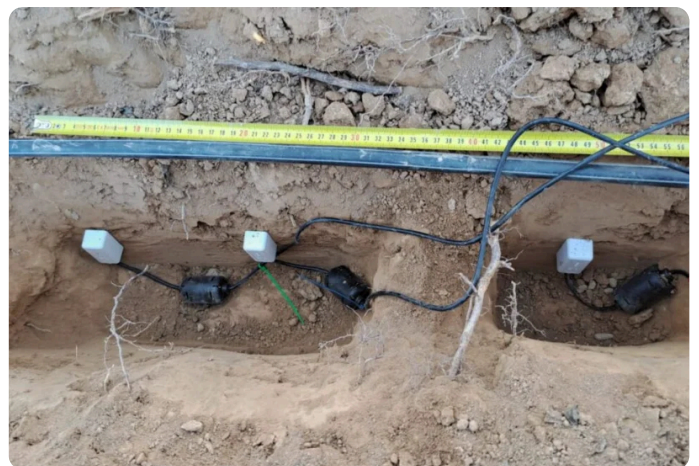
Moisture probes installed in the soil of a productive orchard. Author: Institute of Agrifood Research and Technology (IRTA). © Educational use, non-commercial.
