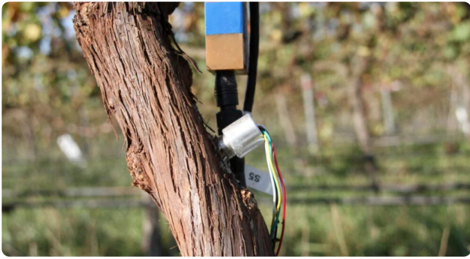
Grapevine with a sensor to measure its hydric status in the form of water potential. Author: Institute of Agrifood Research and Technology (IRTA). © Educational use, non-commercial.
